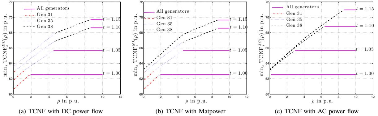
Fig. 5: The lower envelope of TCNF, i.e.,  $\min_s \text{TCNF}_s$  for selected generators in the IEEE 39-bus system.
